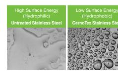
Once applied to the stainless steel it is thermally cured to densify the coating. The resulting coat has a low surface energy (hydrophobic); this makes the moisture from fingerprints less adherent and therefore more easily removed.
